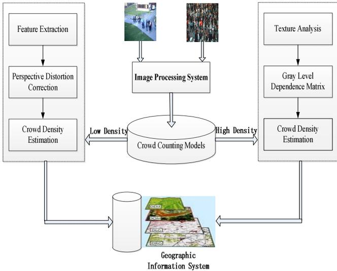
FIGURE III. DATA FLOW DIAGRAM OF REAL-TIME SPATIAL-TEMPORAL ANALYSIS SYSTEM FOR CROWD COUNTING
